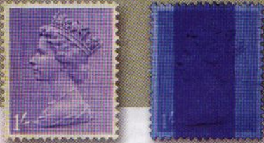
Figure 5. A 1-shilling Machin definitive under normal light (left) and revealing two vertical phosphor bands when exposed to ultraviolet light (right). Sensors on automatic mail sorting machinery detect the phosphor glow.
